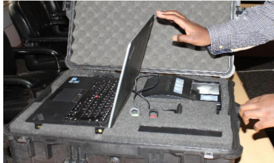
Fig 1: BVR Kit consisting of a laptop, a finger-print scanner and a mountable camera to capture a facial scan.
